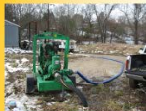
City of Campton's Swift Road well, adjacent to a city lift station. Generator powers pump in well in foreground, overflow is pumped to creek in background.
